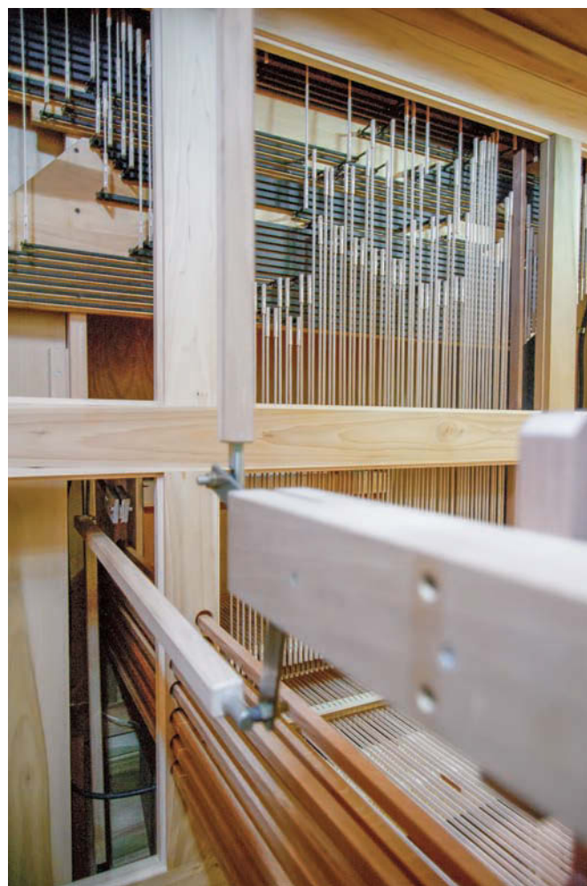
Great key-action roller board, Swell shade mechanism, and Pedal stop action
