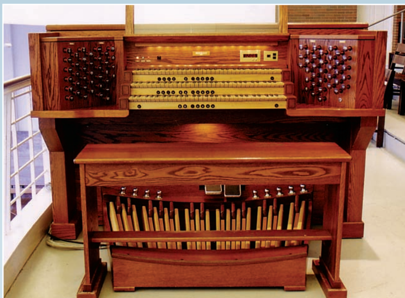
Left: the console is easily moveable. Above: the large Swell and Pedal divisions. Below: the Great and Positiv divisions of the Berghaus organ at the parish of Saint Raphael the Archangel.
